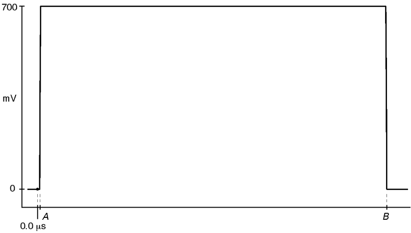
Figure 31: Active Picture Markers, vertical limits, Y channel only
